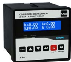
X30-OCEF-240AD (49RMS, 50P, 50N, 51P, 51N, CLP, 50BF, 74TC)
